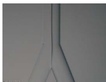
Fig 2. Single Y type microchip (ICC-SY05) with microchannel 100\mu m wide, 40\mu m deep and 4 cm length provided by IMT(Institute of Microchemical Technology Co., Ltd), which is made of borosilicate glass.
