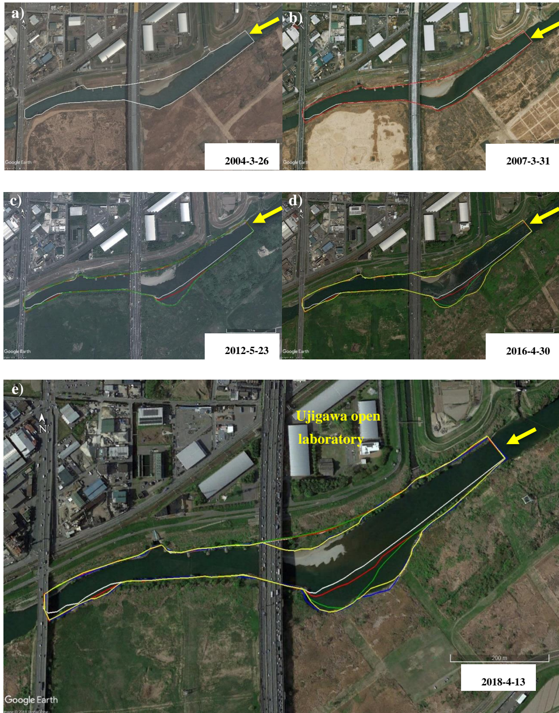
Photos 4.2 (a-e) Bankline change due to the erosion of banks
