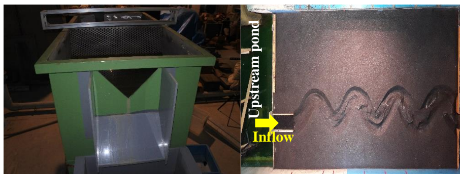
Photo 2.4 V-notch weir for water discharge control
