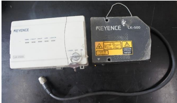
Laser displacement sensor
