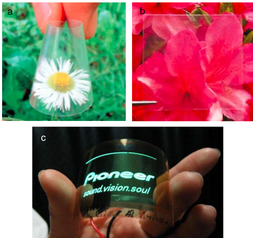
Figure 1.6. (a) A bacterial cellulose nanofiber (BC)-reinforced acrylic resin nanocomposite [1], (b) a wood-CNF-reinforced acrylic resin nanocomposite [67], (c) an organic light-emitting diode (OLED)-display fabricated on a flexible, low-CTE and optically transparent wood-CNF/acrylic resin nanocomposite [74]. Reproduced with permission from (a) ref. 1 © 2005 John Wiley and Sons, (b) ref. 67 © 2005 Springer Nature, and (c) ref. 74 © 2009 Elsevier.
