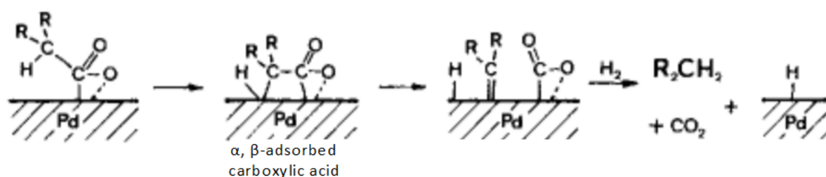
Figure 1-6 The mechanism of C-C bond cleavage in decarboxylation of carboxylic acid [138].
