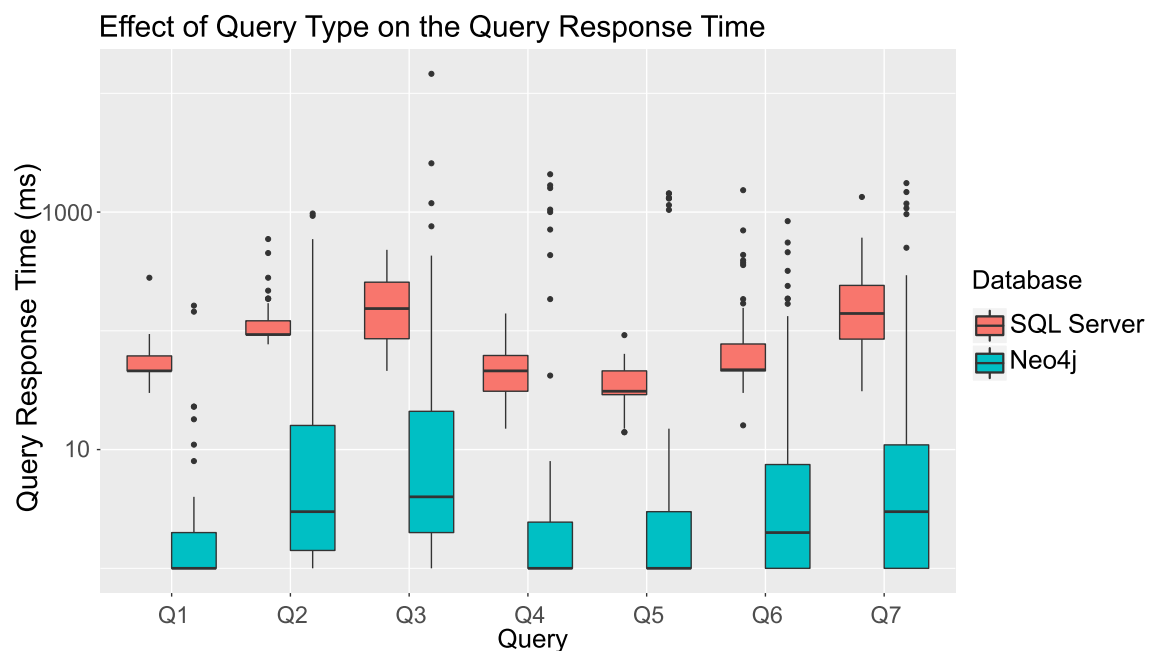
Fig. 7.13: Comparison of the query response times for the two implementation approaches with different queries
