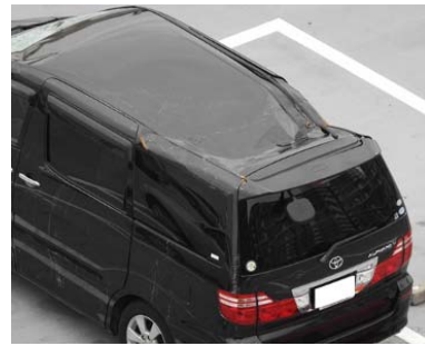
Fig.37 vehicle damage due to flying debris (科研費報告書, 2019)
