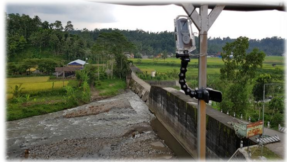
Photo 5 An interval camera monitoring in Lekso river.
