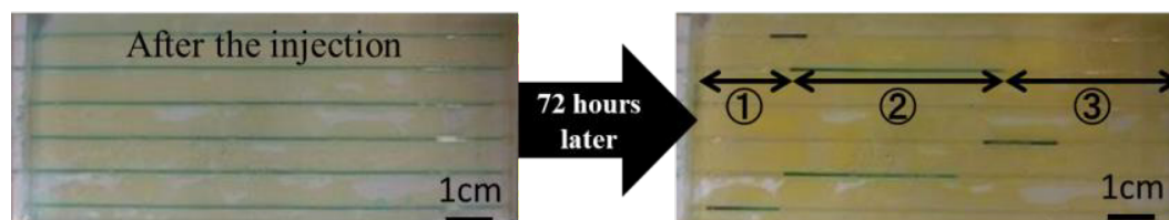
Fig. 2 Solution distribution under conditioning at 74%RH with 60°C ① Gas phase in opened side, ② Solution (Liquid phase), ③ Gas phase in closed side)
