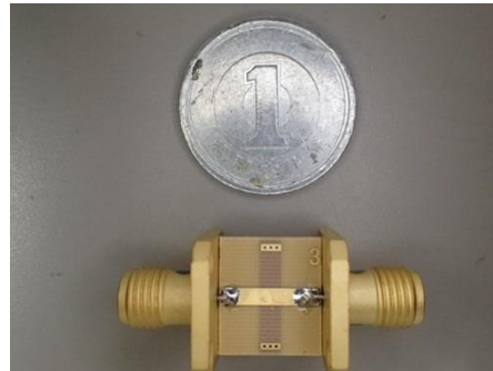
Fig. 2 Developed output filter
