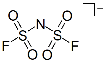
Figure 1-3 Structure of bis(fluorosulfonyl)amide anion ( FSA^- ).
