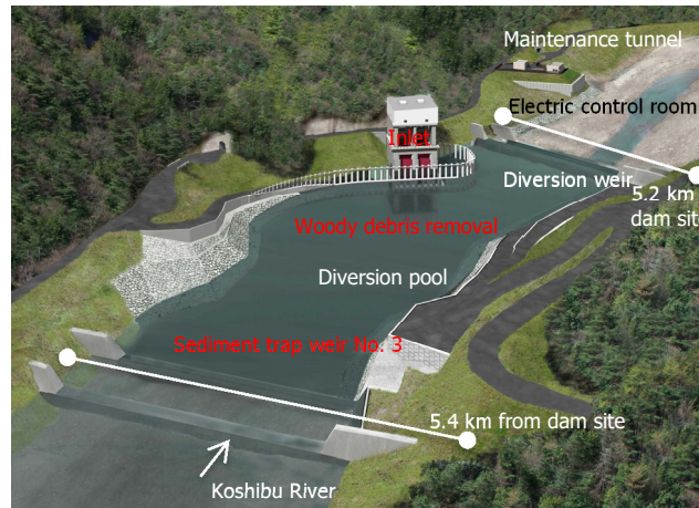
Figure 4: Layout of inlet structure
