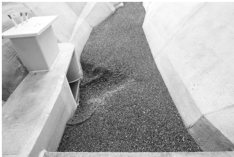
Fig. 12: River bed morphology in the upstream reservoir reach after the flushing test with Q_{SBT} = 200 m 3 /s showing an armouring layer. Only a flushing cone of limited size is scoured out in front of the SBT inlet. (from VAW 2016).
