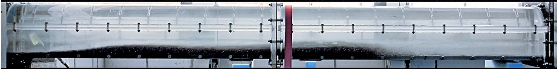
Fig. 13: Side view of the SBT during drawdown with Q_{SBT} = 400 \text{ m}^3/\text{s} like for annual flushing. A dune-like bed form is transported along the tunnel during the drawdown of the reservoir with pressurized flow conditions. The sediment material comes from the deposit in front of the SBT intake which is scoured out by the flow creating a flushing cone (from VAW 2016).
