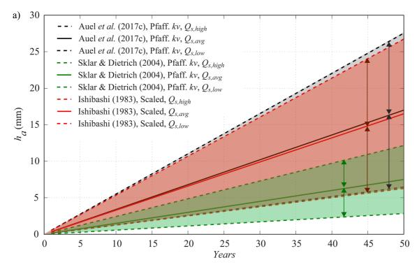
Figure 3: Estimated spatially averaged abrasion depths of Mud Mountain SBT invert lined with Hardy Island Granite versus years of tunnel operation for average abrasion conditions. Sediment load entering the tunnel is  $Q_s = 49,500$  tons/year. Dashed lines correspond to  $\pm 62\%$  of  $Q_s$ . Annual abrasion depths obtained from different models are listed in Table 2.
