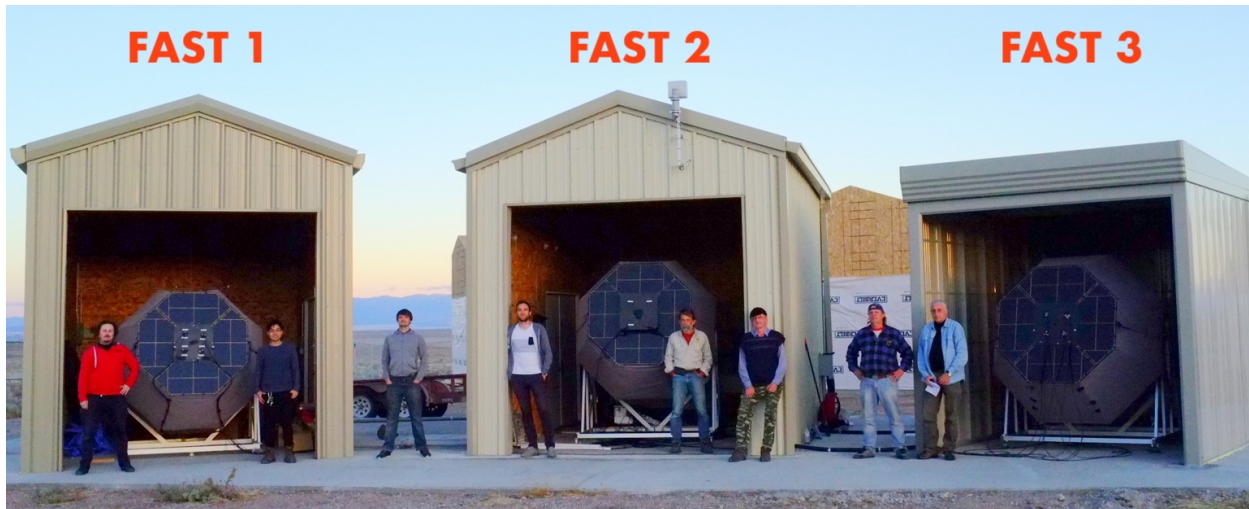
Figure 6: The three FAST prototype telescopes installed at the Black Rock Mesa site of the Telescope Array experiment in central Utah, USA. The FAST All-Sky Camera (FASCam) and Sky Quality Monitor (SQM) can be seen attached to the roof of the central building (see Section 3.5).
