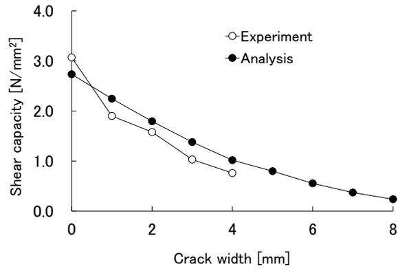
Figure 16 Relationship between joint aperture and shear capacity
