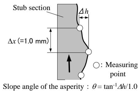
Figure 12 Slope angle of an asperity
