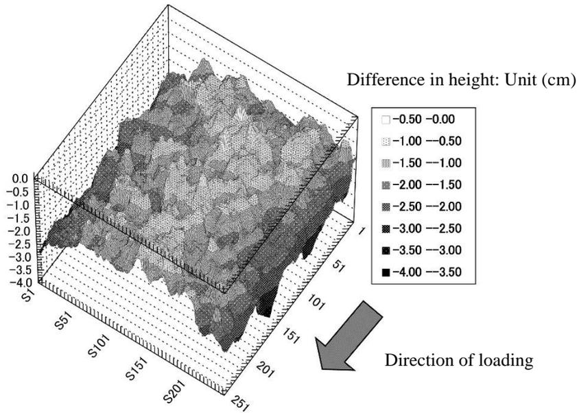
Figure 7 Measured roughness of joint surfaces
