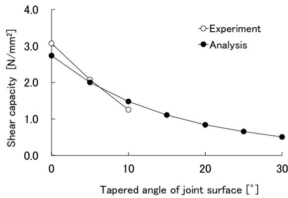
Figure 17 Relationship between tapered angle of joint surface and its shear capacity
