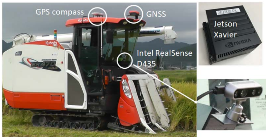
Fig. 4. Robotic combine harvester and devices installed.
