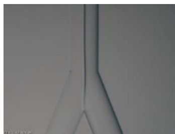
Fig 2. Single Y type microchip (ICC-SY05) with microchannel 100 μm wide, 40 μm deep and 4 cm length provided by IMT(Institute of Microchemical Technology Co., Ltd), which is made of borosilicate glass.
