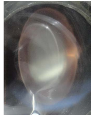
Fig. 2. Solid hydrogen in the target cell
