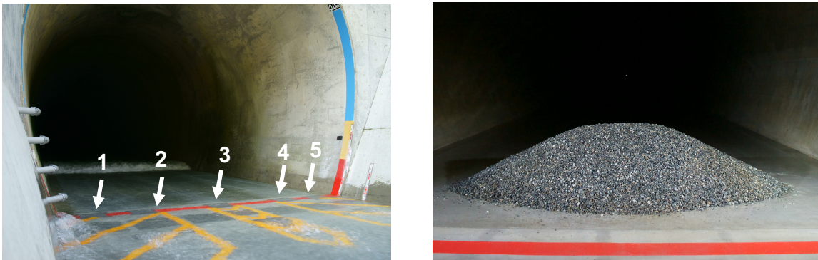
Fig. 4.4 Photos taken during the on-site experiment at the Koshiibu SBT. a) Koshiibu SBT outlet. White arrows show the impact plates, b) Input sediment ( D_s = 10 mm, V = 5 m 3 /s).
