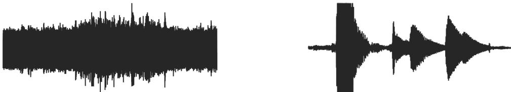
Fig. 5.1 Signals with noise. Left : Signals hindered by water noise, D_s = 2 mm, W = 50 g, and V = 4.5 m/s. Right : Signals with overlapping and saturation. D_s = 100 mm, and V = 4.5 m/s.
