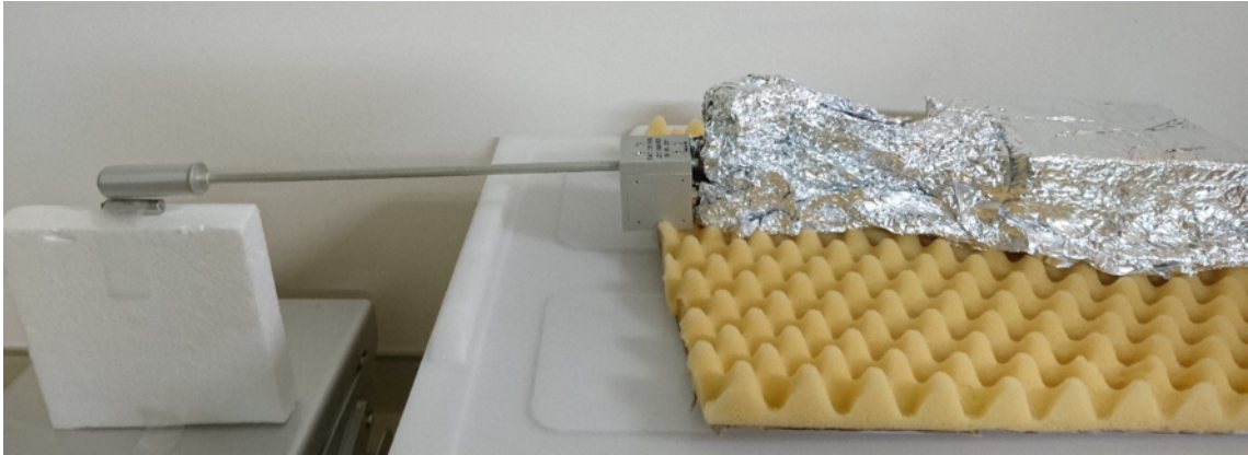
Figure 3.7: Image of the ^{252}\text{Cf} spectrum measurement using LET-1/2 detector.
