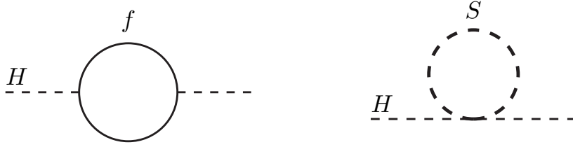
Figure 1.3: The diagrams for one-loop quantum corrections to the Higgs squared mass parameter m_H^2 , due to a Dirac fermion f (left), and a scalar S (right).
