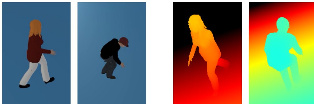
Figure 5. Simulation of human depth maps: (left) two examples of human models inside the simulator performing different actions; (right) the corresponding depth maps from a simulated Kinect sensor (showing just the part of the depth map close to the model).
