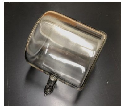
Fig. 3. ^3\text{He} cell (Sekichiku) fabricated at J-PARC.
