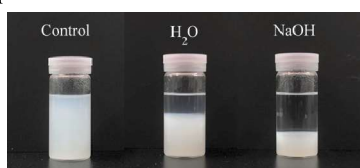
Figure 2. CNF suspension cooked at 160°C for 1 hour with water and alkaline respectively
