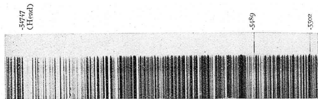
Fig. 1. Absorption of Iodine Vapour at ord. Temp., Magnification : 3.3, 2.3 Å per cm.
