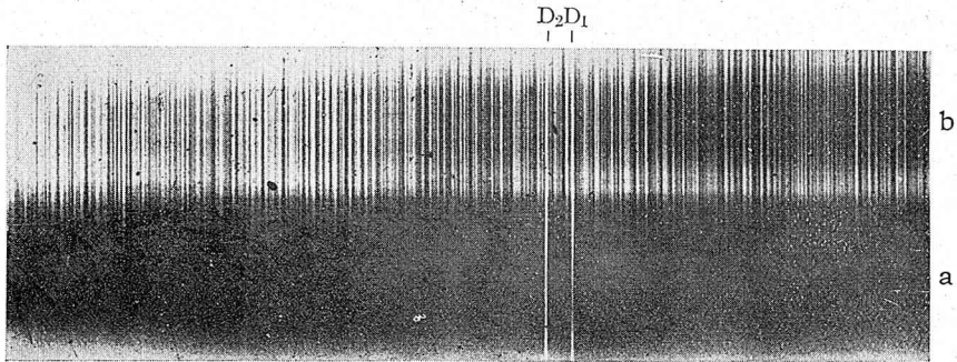
Fig. 2. a: Absorption at ord. Temp., d: 2.5 m. P: 1 atm. 10-foot Concave Grating, b: " at high Temp. D-line Region. 2nd Order.
