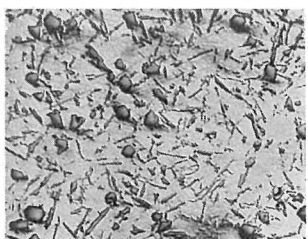
Fig. 12.—Modified with 0.5% Te. \times 100
