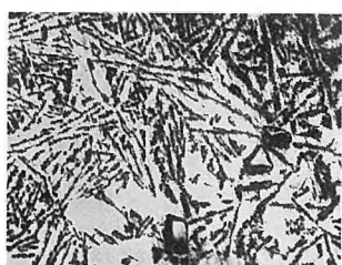
Fig. 15.—Modified with 0.5% Sb. \times 100
