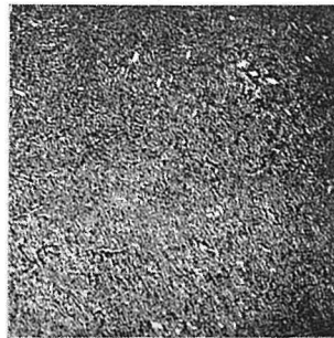
Photo 19. Modified with 0.1% Ca \times 100
