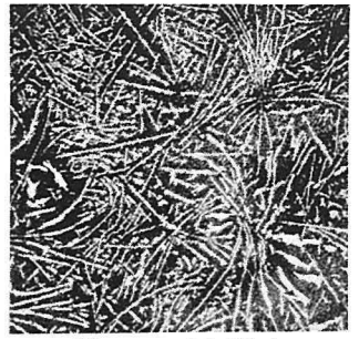
Photo 3. Modified with 0.3% Na \times 100
