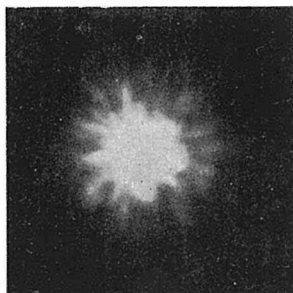
Photo 35. Modified with 0.3% Na. (Transversal section)
