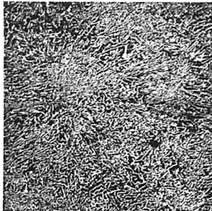
Photo 7. Modified with 0.3% Cd \times 100
