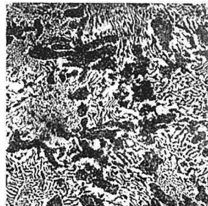
Photo 8. Sn (42%)-Bi alloy. Sand cast \times 100
