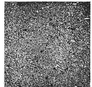
Photo 23. Sb (12.5%)-Pb alloy (H 2 -treated) \times 100
