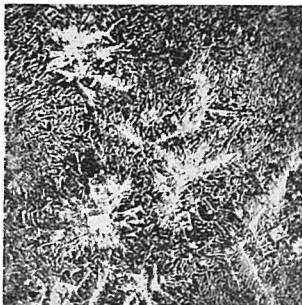
Photo 24. Modified with 0.2% Al (H 2 -treated) \times 100
