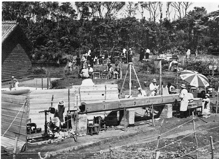
Fig. 2. Whole view of our photographic instrument to observe the annular eclipse. A horizontal long tube, seen on the front side, is the photographic telescope. A coelostat system and objective lens are seen to the left end of the tube, and a focal plane shutter and plate-holder are put to the right end of the tube, shaded by a beach parasol from direct sun-shine.
