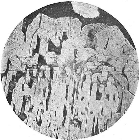
Fig. 5. An honey-combed structure of plagioclase, illustrating that a phenocryst was formed by accumulations of minute ones. (No. 341091, Shin-Také, Kuchierabu-Jima.) (Diam. 0.5 mm.)
