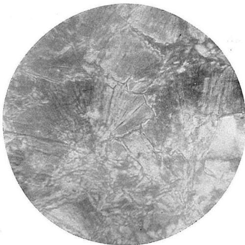
Fig. 29. Large shaped pyrophyllite flakes associated with diaspore, and from 50 to 13.4 microns in length, \times 310 , (crossed nicols).
