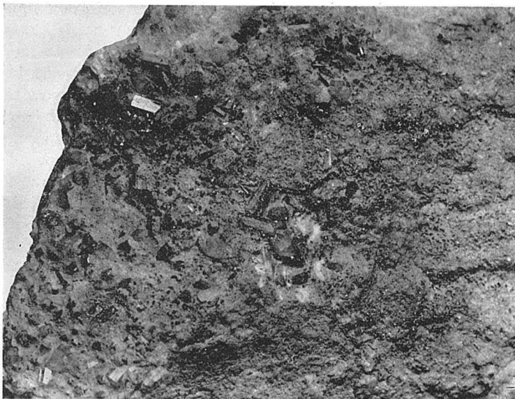
Fig. 25. The diasporite crystals growing on the wall of the druse in coarse grained Tokusyu-Rōseki. One half of the crystal was transformed into the grained part of the Rōseki, and no perfect crystal was isolated from it, \times 23/18 , (from the 2nd gallery at Mituisi Rōseki Company's Mine).
