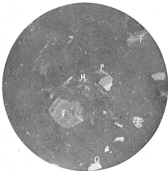
Fig. 5. Liparite from Ikegami gallery (comparatively fresh sample, but a part of the feldspar was altered into pyrophyllite and hydrargillite flakes), \times 50 , (crossed nicols).
