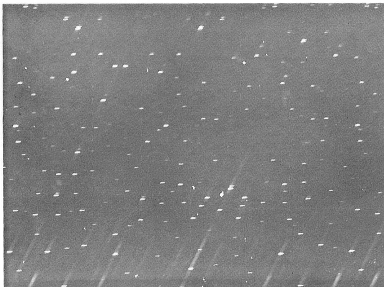
Fig. 2. A Weissenberg photograph of Ti-oxyhornblende about the c-axis (zero level)
