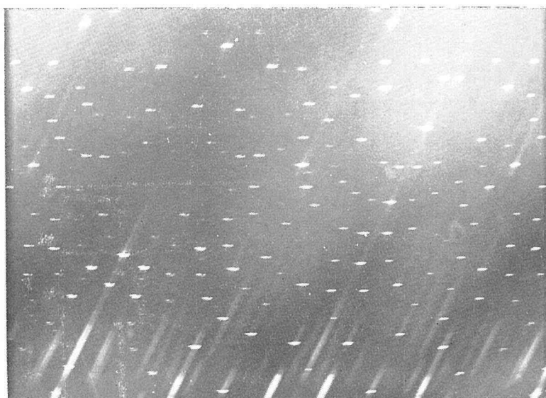
Fig. 2. B Weissenberg photograph of the oxyhornblende about the c-axis (zero level)
