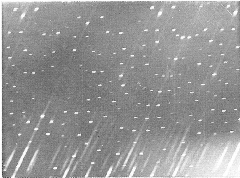
Fig. 10. (A) Weissenberg photograph of actinolite about c-axis. (zero level)
