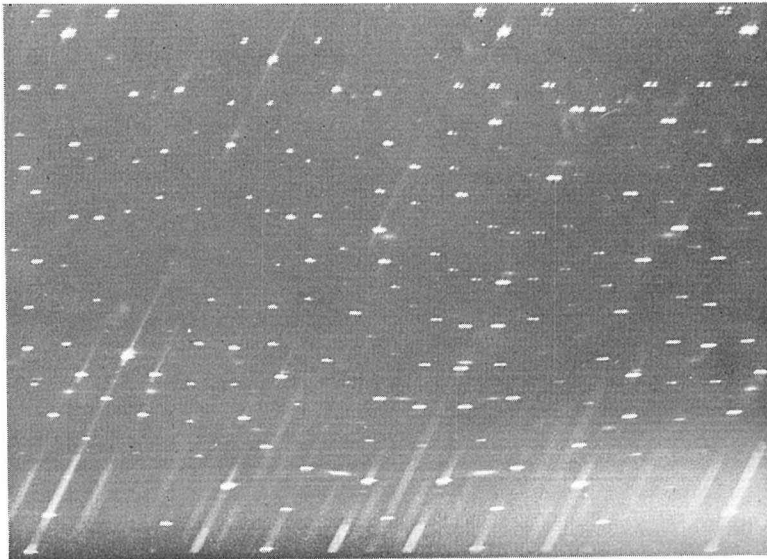
Fig. 8. (B) Weissenberg photograph of tremolite about c-axis, heated at 900°C for 2 hours. (zero level)
