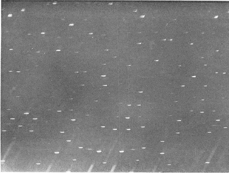
Fig. 10. (B) Weissenberg photograph of actinolite about c -axis, heated at 900^{\circ}\text{C} for 2 hours. (zero level)
