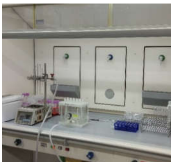
Fig. 3.1 Sample extraction using SPE vacuum manifold
