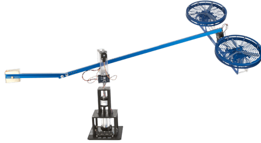
Figure 5.5: Quanser’s 3 DOF helicopter ( https://www.quanser.com/products/3-dof-helicopter/ ).
