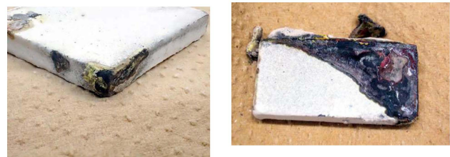
Fig. 2. In the second MT, over heat was assumed and some liquid metal was over spilled from the container.
