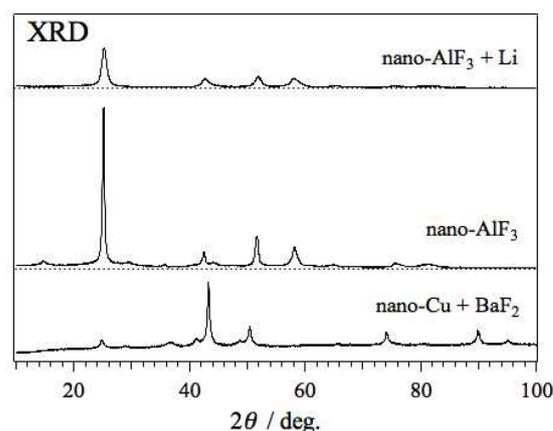
Fig. 2. (a) Neutron diffraction data of Cu nanoparticle with BaF<sub>2</sub> (nano-Cu + BaF<sub>2</sub>), AlF<sub>3</sub> nanoparticle (nano-AlF<sub>3</sub>), AlF<sub>3</sub> nanoparticle with Li (nano-AlF<sub>3</sub> + Li) collected at the VCND. (b) X-ray diffraction data of the “nano-Cu + BaF<sub>2</sub>”, the “nano-AlF<sub>3</sub>”, and the “nano-AlF<sub>3</sub> + Li” collected at the X-ray diffractometer with CuK $\alpha$  radiation.
