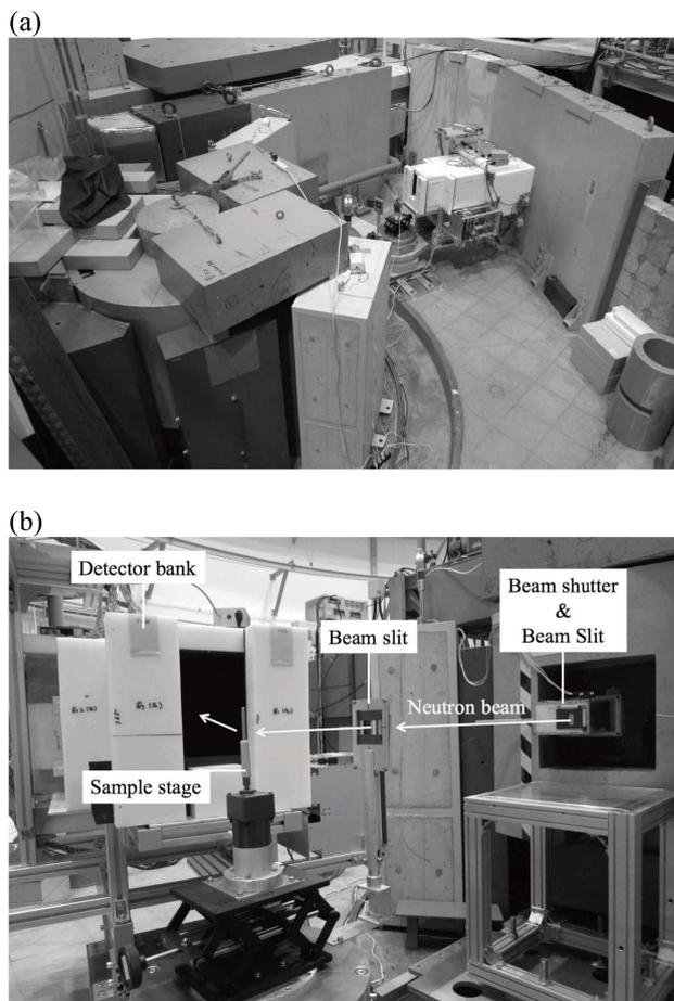
Fig. 1. Versatile compact neutron diffractometer (VCND) installed at the B-3 beam port of Kyoto University Research Reactor (KUR): (a) bird's-eye-view photograph and (b) partial view (around the sample stage) of the VCND.
