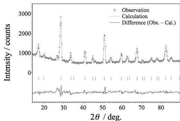
Fig. 2. The crystal structure refinement of  $\text{SrF}_2$  using neutron diffraction data collected at the VCND.
