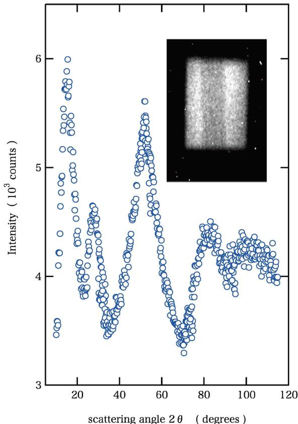
Fig. 1. Neutron diffraction pattern of the borosilicate glass for vitrification without simulated radioactive waste recorded on the B-3 diffractometer. The inset shows a neutron transmission image for the same sample.
