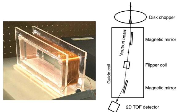
Fig. 1. New flipper coil with large acceptance.
