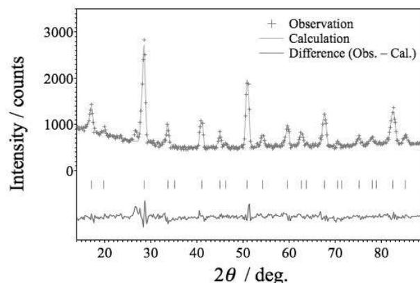
Fig. 2. The crystal structure refinement of SrF<sub>2</sub> using neutron diffraction data collected at the VCND.
