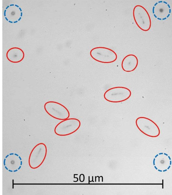
Fig. 1. Microscopic image of the detector after development. Observed tracks are surrounded by red ellipses. Marks for fine alignment are surrounded by dashed blue circles. Tracks and marks were clearly seen after development.
