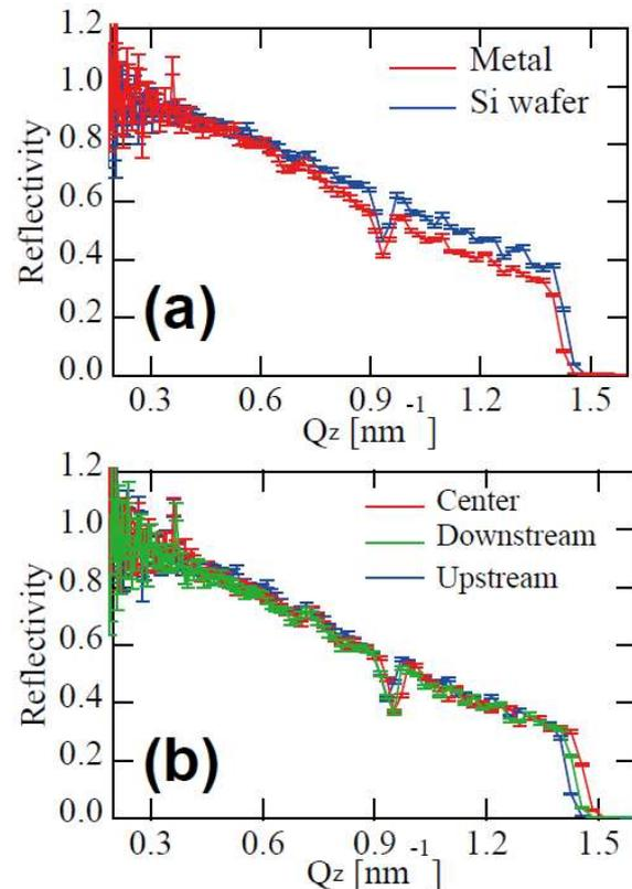
Fig. 1. Neutron reflectivity of  $m=6.5$  NiC/Ti (SiC) supermirror deposited simultaneously on (a) metal substrate and silicon wafer. (b) Those on different metal elements (upstream, center downstream parts).
