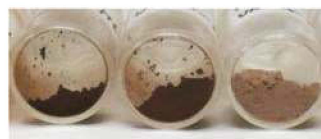
Fig. 1. Typical appearance of simulated MCCI debris prepared under reducing conditions.
