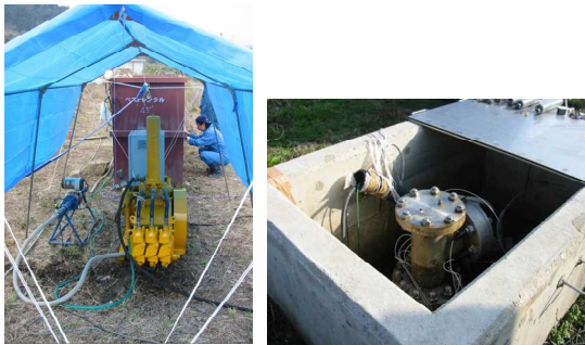
Photo 7. Water injection experiment into the 1700m bore-hole at the Ogura site of the Nojima fault.
