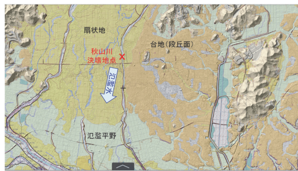
Fig. 4 Land-type map at the downstream part of the Akiyama River (based on GIS map). Levee breaching occurred at the fluvial fan and the flooded water was ponded on floodplain in the downstream part.
