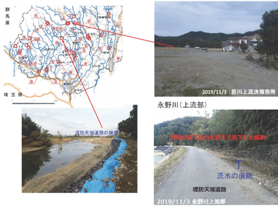
Fig. 6 Levee breaching and overtopping points along the Nagano and Omoi rivers (photos are taken by the author on Nov. 3, 2019)
