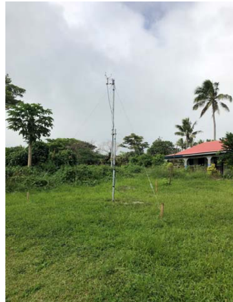
Photo 1 Ultrasonic anemometer installed in Vanuatu
