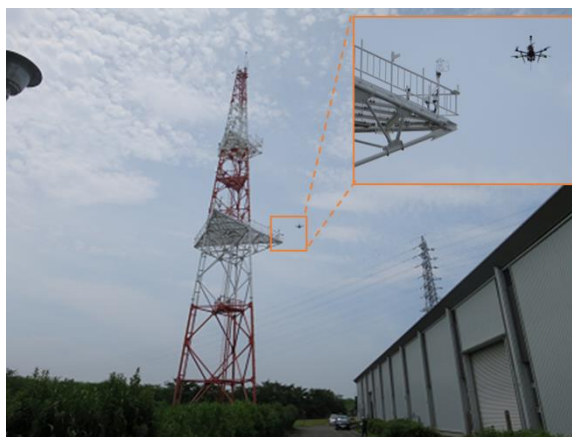
Fig. 11 Hovering drone at Site B nearby meteorological observation tower equipped with ultra-sonic anemometer.
