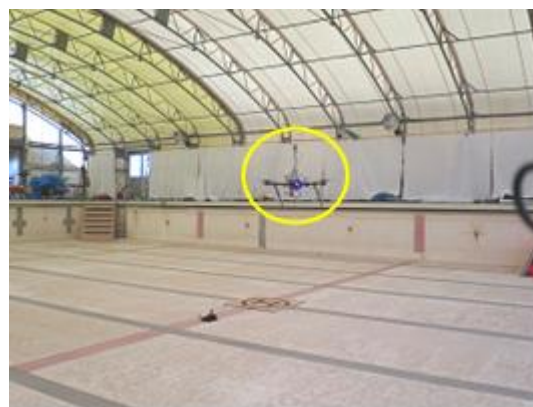
Fig. 3 Hovering drone installed with ultra-sonic anemometer at 2 m from floor.
