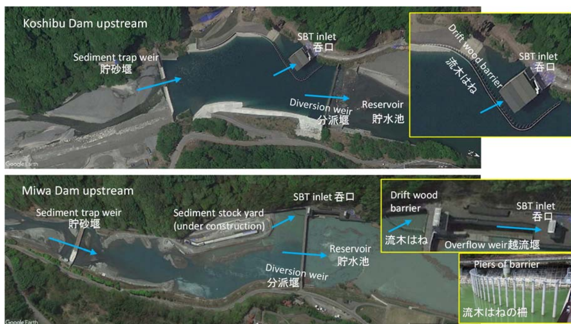
Fig. 1 Plan view of upstream SBT structures in Koshibu and Miwa Dams. Images by Google Earth.
