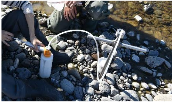
Fig. 16 Hyporheo sampler of suck-up type with a strainer and a hand pump (produced by T. Torii).
