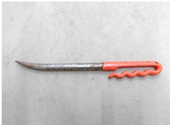
Fig. 12 Survey tool for riverbed softness
