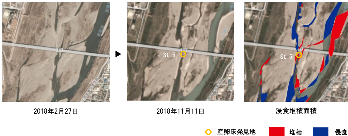
Fig. 31 Erosion deposition area (Right bank sand bar at from 14.2 km to 9.3km)
