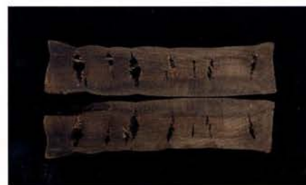
Honeycombs of Acacia mangium, a quick test of 100°C
