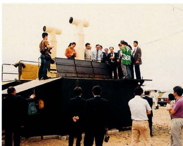
The inspectors and press men were confirming the odorless operation of the livestock manure fermenters (LMFs), containing 8m 3 sawdust as an artificial soil matrix. Pig manure (0.5 t/day) has been composted without formation of odor for 20 days.
