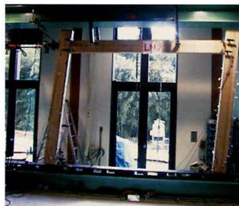
An image of the portal frame made of LVL subjected to a push-pull cyclic lateral loading for evaluating structural performance of beam-column joints. (Photo. 2)
