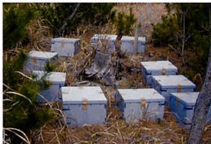
Field test for wood degradation at a site infested with termites
