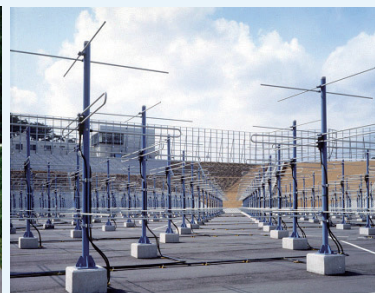
MU radar antenna the first large-scale MST radar with a two-dimensional active phased array antenna system Completion: 1984 Size: 103 m in diameter Award: selected as IEEE Milestone
