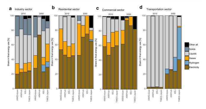
Fig. 4 Share of fuels in final energy by sectors in 2010 and 2050 in 26by30+80by50\_Def: a Industry sector, b Residential sector, c Commercial sector, and d Transportation sector
