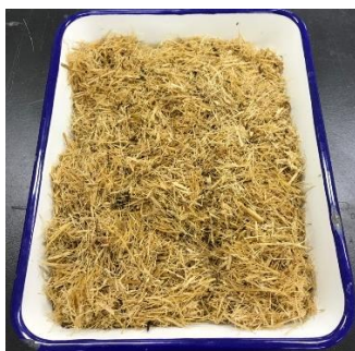
Figure 3.4 Bagasse fibers after the alkali treatment
