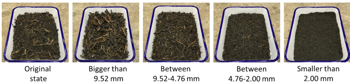
Figure 3.8 The original state and the sieved burned bagasse
