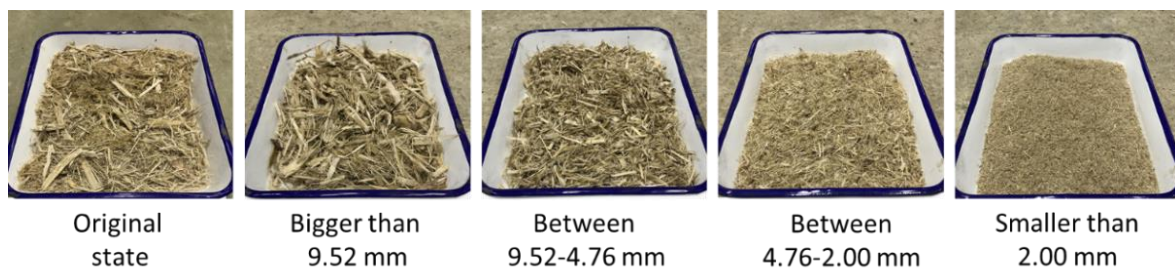
Figure 3.3 Original state and the sieved bagasse fiber
