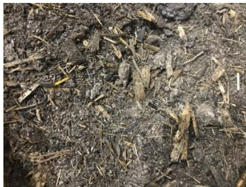
Figure 2.9 Residual sand and ash with the presence of non-burned bagasse
