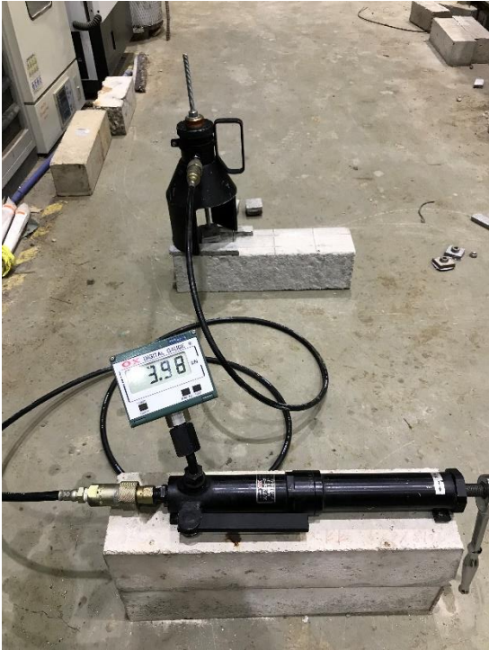
Figure 4.4 Overview of the adhesion strength test
