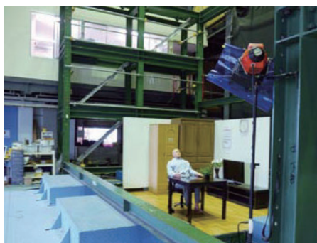
強震応答実験装置 Strong earthquake response simulator
