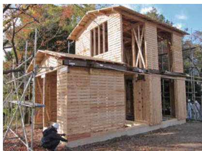
実大木造家屋引き倒し実験による『壁柱』耐震補強方法の検証 Validation of seismic reinforcement by the so-called "Column-Wall" by pull-down experiment of real size wooden houses
