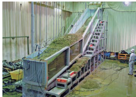
室内降雨崩壊実験（森林総合研究所の施設を利用） Flume experiment related to rainfall induced shallow landslides (used the equipment in Forestry and Forest Prod. Res. Inst., Tsukuba)
