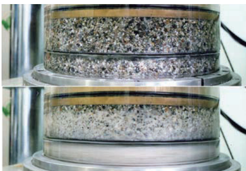
高速せん断中に発生した粒子破砕現象 Particle crushing during high-speed ring shear test
