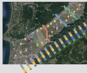
島知漏平野における微動観測点配置図と推定した地盤構造断面図(google mapに加筆) Microtremor observation stations and estimated subsurface structure section of Ochigata plain (plotted on Google Map).
