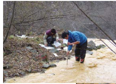
穂高砂防観測所の観測流域における土砂流出時の河床変動計測 Bed level measurement during sediment flushing event in Hodaka observation area.
